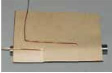
Subsequently, the fishpaper is cut in such a way that the wires in the slots can be led out. The paper is then put to the coil in the respective sense of coil (!) around the magnet and covered with the coil.
